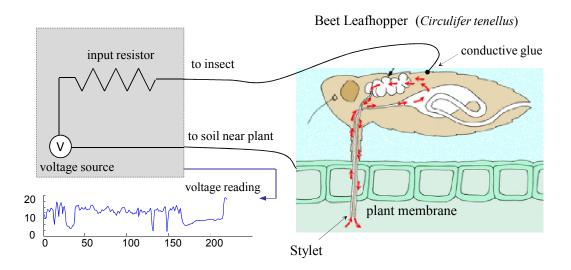
Figure 2.16: A schematic diagram showing the apparatus used to record insect behavior
