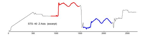
Figure 4.1: Forty-five minutes of Space Shuttle telemetry from an accelerometer. The two occurrences of the best ten-minute long motif are highlighted
