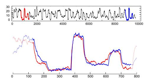
Figure 1.1: (*top*) The output steam flow telemetry of the Steamgen dataset has a motif of length 640 beginning at locations 589 and 8,895. (*bottom*) by overlaying the two motifs we can see how remarkably similar they are to each other.
