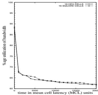
Figure 4: Effect of shape on utilization: 18 hexagonal vs 16 square cells
