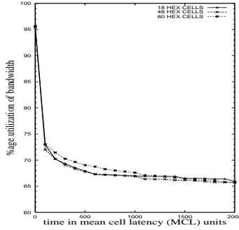
Figure 3: Variation of utilization with network size: 18, 48, and 80 hexagonal cells
