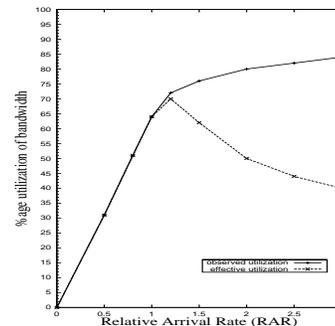
Figure 1: Observed and effective utilization vs. relative arrival rate
