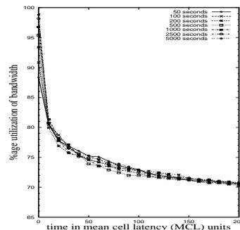
Figure 2: Variation of utilization with cell latency : 48 hexagonal cells
