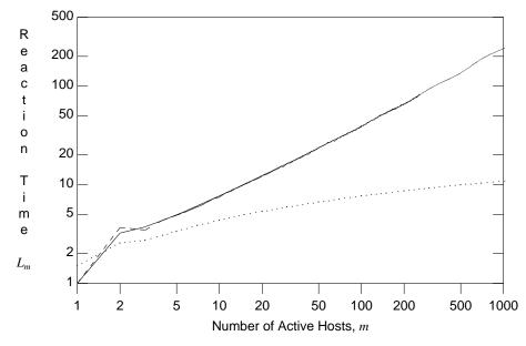
Figure 7: Average time to the first successful transmission after the "Big Bang", starting from m active hosts. Solid line is from Eq. (5), which is approximate because of an independence assumption. Dashed line is the sample mean obtained by Monte Carlo simulation of the exact system. Dotted line is from Eq. (6), which is the equivalent result for the Binary Logarithmic Arbitration Method that will be introduced in section III.
