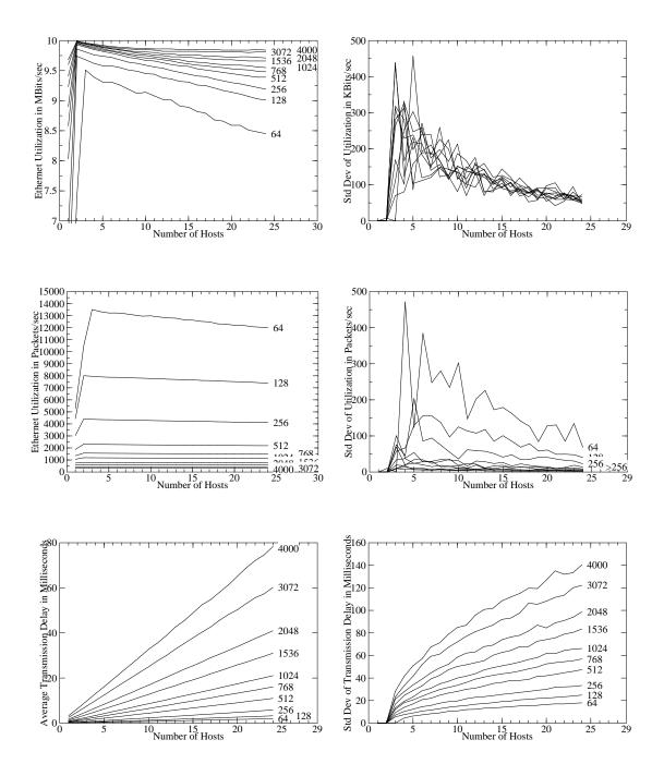
Figure 1: Published measurement data on Ethernet performance under overload conditions. Graphs shown above correspond to Figures 3-3 through 3-8 from [6], in top-to-bottom, left-to-right order, and are copyright 1988 by Digital Equipment Corporation. Used by permission.
