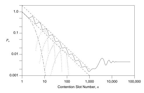
Figure 6: Network load drops off slowly after the "Big Bang". Solid line indicates the probability,  $P_n$ , that a given host will attempt a retransmission in the *n*th backoff slot, assuming none of its earlier attempts were successful. Dashed lines bounding  $P_n$  are the harmonic functions 1/n and 2/n, respectively. Dashed line at lower left is the geometric function  $1/2^n$ . "Arch" shaped dotted lines show, from left to right, the component functions  $P_n(3), \ldots, P_n(6)$ .
