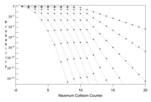
Figure 18: The probability distribution function,  $F_{CC}(k)$ , for the collision counter of a departing packet under BLAM, conditioned on *M*, the number of hosts currently active. (Curves from left to right correspond to M = 2, 4, 8, 16, 32, 64, 128, 256, 512, 1024.)
