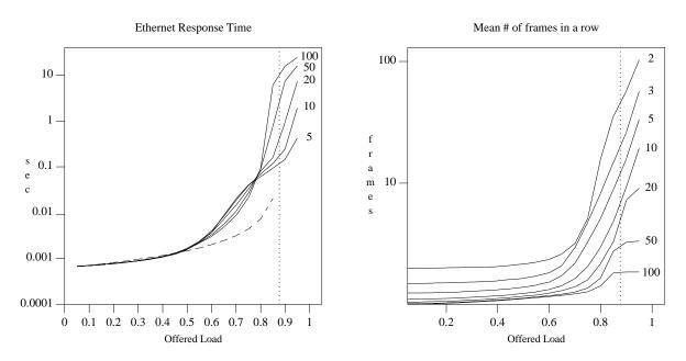
Figure 5: Effect of Number of Active Hosts on Ethernet Response Times (including both waiting time and access time). Solid lines: simulation data by Armyros [5]. Dashed line: approximate analytical formula due to Almes and Lazowska [4], which is based on the simplistic capacity analysis in [21]. Dotted line: predicted capacity using Almes and Lazowska's formula, which ignores the capture effect.
