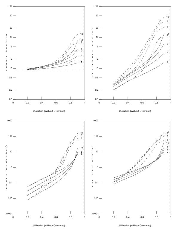
Figure 14: Comparison of the Mean and Standard Deviation of the Access Time and Queueing Delay between the Standard Ethernent and the Binary Logarithmic Arbitration Method, assuming 1024 byte packets, symmetric Poisson arrivals, and various numbers of hosts. Network topology follows the experimental setup in [6]. Dashed lines represent a system with only Standard Ethernet hosts, while solid lines represent the same system using BLAM.
