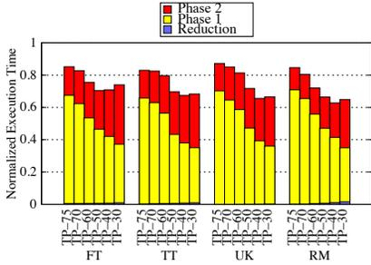
(d) Normalized Execution times for GC. For comparison, the Baseline execution times (in sec) for FT, TT, UK and RM are 1216, 1014, 771 and 33.51 respectively.
