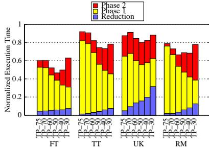
(a) Normalized Execution times for SSSP. For comparison, the Baseline execution times (in sec) for FT, TT, UK and RM are 127.14, 96.15, 4.65 and 2.71 respectively.
