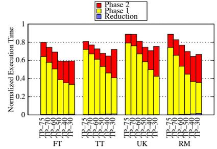
(f) Normalized Execution times for CD. For comparison, the Baseline execution times (in sec) for FT, TT, UK and RM are 1351, 896, 654 and 33.25 respectively.
