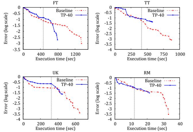
Figure 8: Relative Error (log scale) vs. Execution Time (sec) for CD: Baseline and TP-40. Note that the point at which the Baseline version terminates, i.e., relative error becomes zero, is not plotted due to use of log scale.
