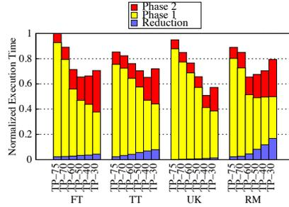
(e) Normalized Execution times for CC. For comparison, the Baseline execution times (in sec) for FT, TT, UK and RM are 264.64, 118.71, 137.6 and 3.05 respectively.
