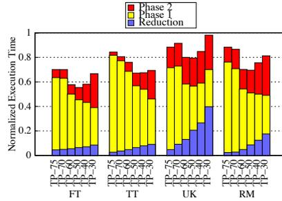
(b) Normalized Execution times for SSWP. For comparison, the Baseline execution times (in sec) for FT, TT, UK and RM are 134.67, 104.32, 4.81 and 2.9 respectively.
