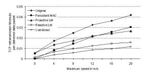
Fig. 6. TCP retransmission time-outs per delivered packet as a function of maximum speed.
