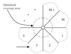
Fig. 1: The circular directional transmission
