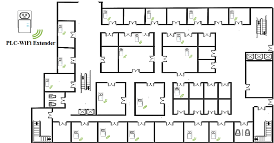
Fig. 1: Powerline communications extend WiFi coverage through existing interior power lines in a home/enterprise.
