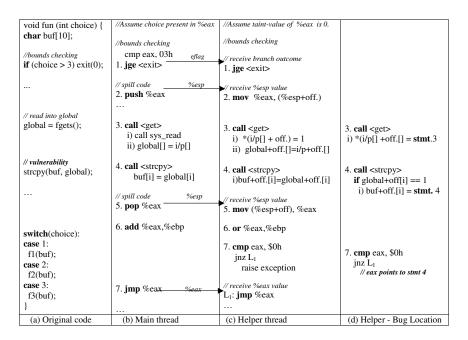
Figure 1: DIFT/Bug Location using helper threads
