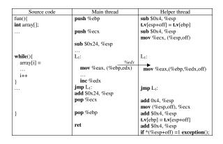
Figure 2: Register indirect Optimization
