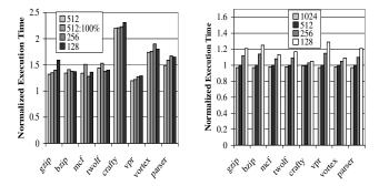
Figure 7: Sensitivity on L2 Cache Size and Queue Size
