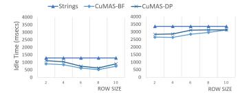
Figure 9: Idle time observed two resource channels: P[GPU] on the left (a) and R[D2H] on the right (b)
