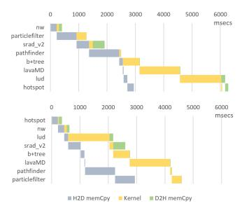
Figure 2: (a) On the top, an overlapping example exploited on a subset of Rodinia applications using a random arrival ordering; and (b) On the bottom, a data transfer-aware re-ordering of the same subset.
