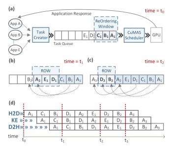
Figure 5: (a) CuMAS task creation, queuing and reordering for different applications at initial time  $t_0$ , (b)  $t_1$ , and (c)  $t_2$ . (d) On the bottom: View of the HW pipeline of tasks after re-ordering.<sup>2</sup>
