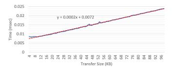
Figure 11: Data transfer times (solid) and corresponding curve fitting (dashed).
