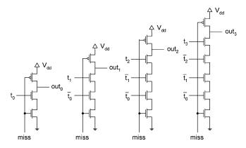
Fig. 22. Single priority selector circuits.
