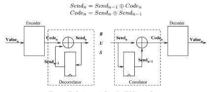
Fig. 4. Reducing switching by XORing values.
