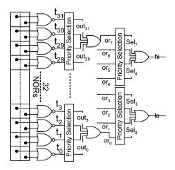
Fig. 23. Timestamp registers and priority selectors circuits.
