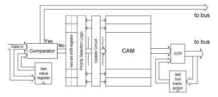
Fig. 20. Encoder components.
