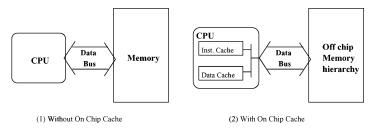
Fig. 18. Architecture models with and without on-chip caches.
