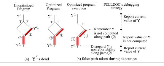
Figure 7.3: Not computed in the optimized program example
