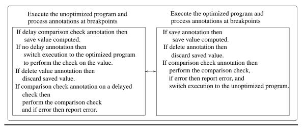
Figure 5.3: Comparison checker algorithm
