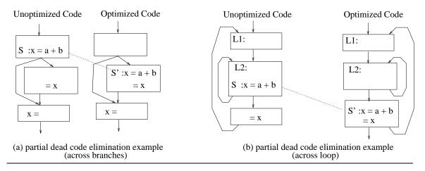
Figure 3.7: Code sinking transformation examples
