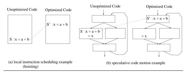
Figure 3.3: Code hoisting transformation examples
