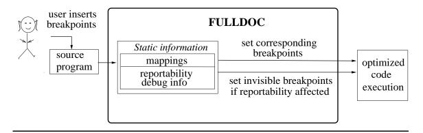
Figure 7.4: FULLDOC's strategy with respect to user inserting breakpoints
