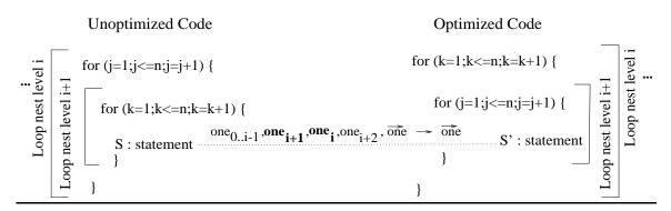
Figure 4.7: Loop interchange effects on initial  $\overrightarrow{one} \rightarrow \overrightarrow{one}$  mappings
