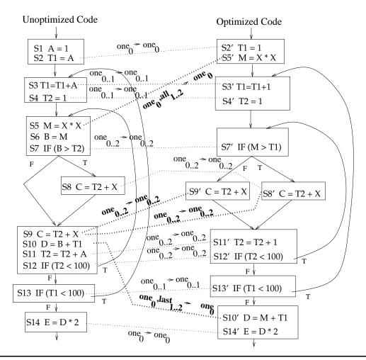
Figure 4.5: Mappings for unoptimized and optimized code example
