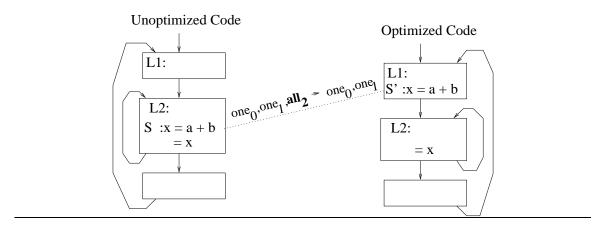
Figure 4.1: Loop invariant code motion mapping example
