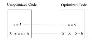
Figure 3.1: Constant propagation example
