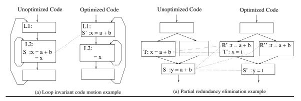
Figure 3.5: Code hoisting transformation examples cont.
