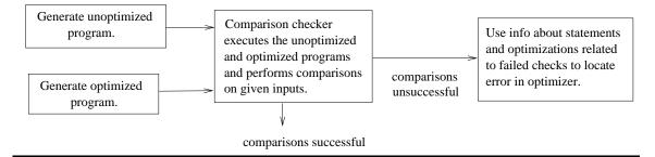
Figure 5.1: The comparison checking system
