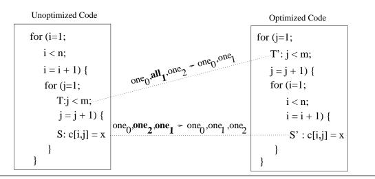
Figure 4.3: Loop interchange mapping example
