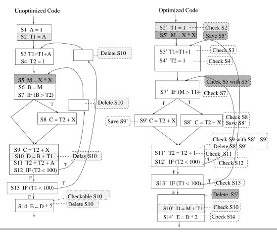
Figure 5.5: Annotated unoptimized and optimized code example
