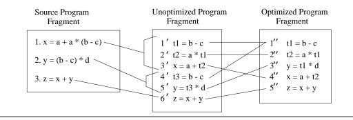
Figure 2.1: Source program and its unoptimized and optimized program versions example
