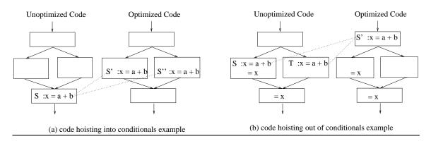
Figure 3.4: Code hoisting transformation examples cont.
