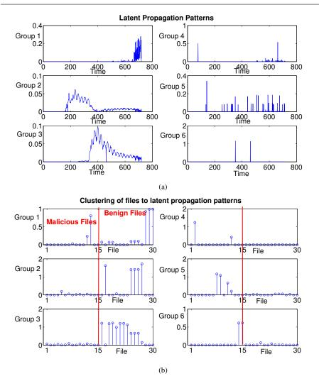
Fig. 11 Latent representation of the propagation pattern, and clustering of the time series, after sampling. In both subfigures, the vertical axis represents the degree of participation of each data point to the particular Group/Co-cluster. In subfigure (a) the horizontal axis is time and in subfigure (b) the horizontal axis is the file ID.
