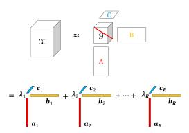
**Fig. 2:** Rank-R PARAFAC decomposition of a three-way tensor. The tensor  $\mathfrak{X}$  is decomposed as three factor matrices  $\mathbf{A}$ ,  $\mathbf{B}$ , and  $\mathbf{C}$ .
