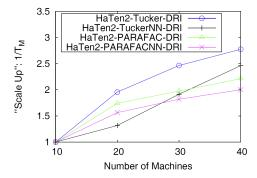
Fig. 10: Machine scalability of HATEN2-PARAFAC-DRI, HATEN2-PARAFACNN-DRI, HATEN2-Tucker-DRI, and HATEN2-TuckerNN-DRI with regard to the "Scale Up" factor  $\frac{T_{10}}{T_M}$ , where  $T_M$  is the running time with M machines. Note that in all cases, HATEN2-DRI scales near linearly in the beginning, while the performance flattens as more machines are added due to overheads in distributed systems.
