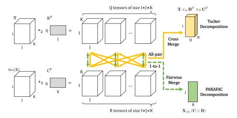
Fig. 4: General computational framework in HATEN2 for Tucker and PARAFAC decompositions (Q=R in PARAFAC). Although the two decompositions are different, our HATEN2 unifies them into a general framework where the two methods differ only at the final merge step: CrossMerge for HATEN2-Tucker, and PairwiseMerge for HATEN2-PARAFAC (see Section 3.2.4 for details).
