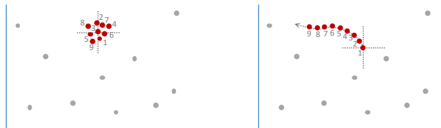
Fig. 1. Visualizing time series subsequences as points in high-dimensional space. left ) A time series motif can be seen as a collection of points that approximate a platonic ideal, represented here as the crosshairs. right ) In contrast, a time series chain may be seen as an evolving trail of points in the space. Here the crosshairs represent the first link in the chain, the anchor .
