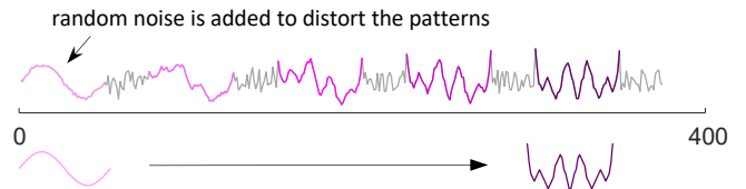
Fig. 14. Synthetic time series embedded with a chain of five subsequences. The subsequences evolve from a sine-wave to a random-walk pattern.
