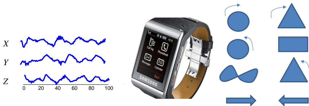
Fig.19 left ) Sample accelerometer data ( X , Y and Z ) of a gesture. middle ) A Samsung Gear 2 used to collect activity data. right ) the eight different gestures considered in our experiments.
