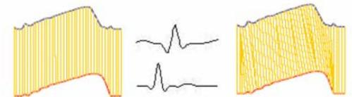
Figure 3. One to one alignment on time axis vs. non-linear alignment (warped time axis). Nonlinear curve alignment is important in pattern recognition of ECG signals. Wavelet analysis dose not allow this type of flexibility in pattern recognition and matching.
