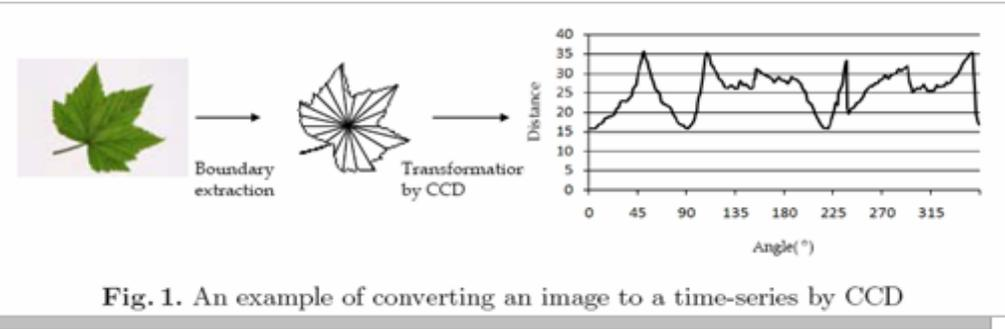
Fig. 1. An example of converting an image to a time-series by CCD
