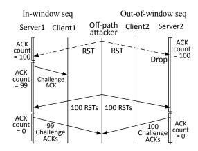
Figure 2: An illustrative TCP Side-Channel Vulnerability.
