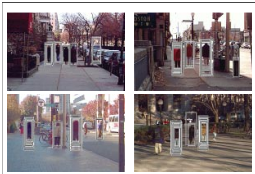
Figure 10: Results from the pedestrian detection system. Typically, missed pedestrians are due to occlusion or lack of contrast with the background. False positives can be eliminated with further training. From Papageorgiou, Evgeniou, and Poggio (1998)
