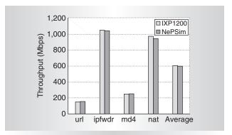
Figure 2. NePSim and IXP1200 throughput comparison.
