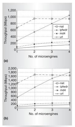
Figure 4. Impact of number of microengines on throughput: four threads per ME at 232 MHz (a), four threads per ME at 464 MHz (b).
