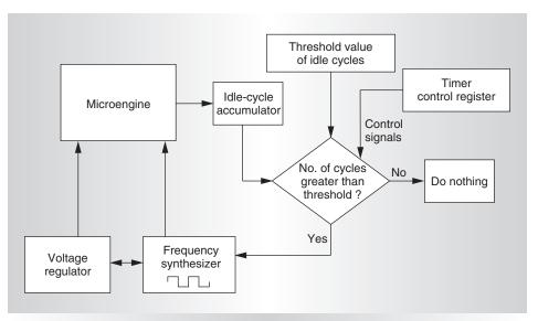
Figure 10. Dynamic voltage scaling (DVS) policy control mechanism.
