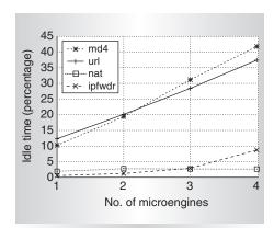
Figure 9. Average core idle time with different numbers of microengines and active threads (four threads per ME at 464 MHz).
